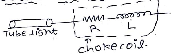
• choke coil can reduce voltage to tube if its impedance Z is high.
