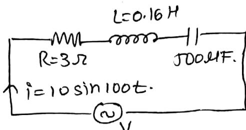
Find:  $\omega$  $X_L, X_C, Z, \phi, V_0, V(t), V_R(t)$  $V_L(t), V_C(t)$ , Power factor.
