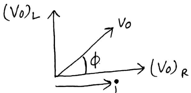
$$\therefore V_0^2 = (V_0)_R^2 + (V_0)_L^2$$
