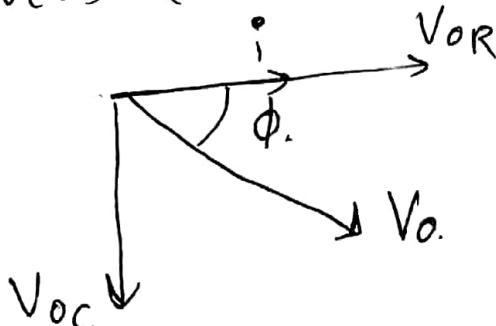
$$V_o = \sqrt{V_{oR}^2 + V_{oC}^2} \quad (11)$$
