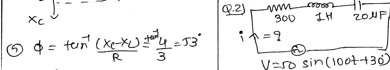
Find  $X_L, X_C, Z, \phi$  $i_0, i(t), V_R(t), V_L(t), V_C(t)$ , power factor & power.
