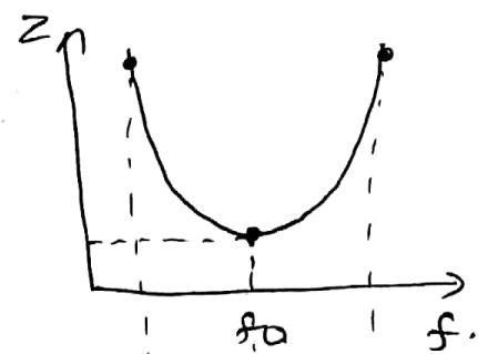
$$\begin{aligned} \therefore z &= \sqrt{R^2 + (X_L - X_C)^2} \\ &= \sqrt{R^2 + (2\pi f L - \frac{1}{2\pi f C})^2} \end{aligned}$$
