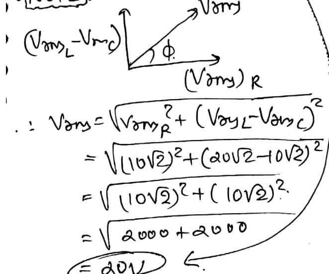
$$\therefore V_{avg} = \sqrt{V_{avgR}^2 + (V_{avgL} - V_{avgC})^2} \\ = \sqrt{(10\sqrt{2})^2 + (20\sqrt{2} - 10\sqrt{2})^2} \\ = \sqrt{(10\sqrt{2})^2 + (10\sqrt{2})^2} \\ = \sqrt{2000 + 2000} \\ = 20V$$
